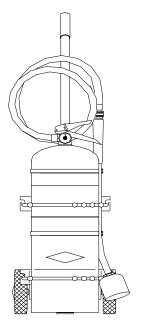
Place the extinguisher into the model 589 dolly and fasten the rubber "bungee" straps around the cylinder. Install the hose and extension applicator into both clips as instructed above (steps 1 & 2). DO NOT INSTALL THE RUBBER STRAPS OVER THE HOSE & APPLICATOR.
